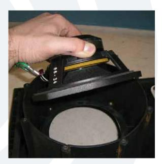
The mid frequency driver easily lifts right off of the horn. Replace with the new driver (part #0013897) and follow the same steps as above, but backwards 7 to 1. Power up the SA1530z and the new driver should now be pumping out those mids again. Right on, you just replaced a mid frequency driver!
